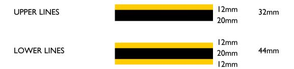
Some of these lines now need to be applied to the coach side in chalk. For the lower lines we will need the top and bottom, the outer limits of the ochre. For the top lines we will just need the top of the ochre.
