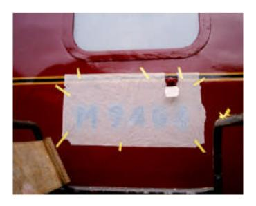
Fix your tracing in position on the coach side using a bit of Cellux tape. Check it's in the right place and horizontal. Then using a pencil and ruler, go over the lines so as to transfer the chalk to the coach.
