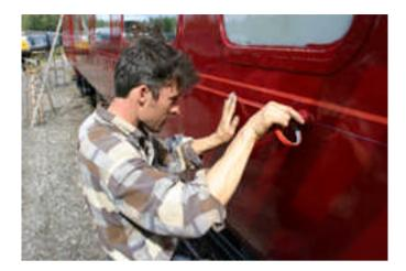
Using the Cellux tape, mask up to the outside of your lines, as demonstrated. At the top just mask up above your single line. Finish the line on the apex of the curve at the end of the coach, and mask the ends also. Rub out any air bubbles near the paint edges, else you will get paint creeping underneath. Dust off any chalk marks once the tape is in place. Note this is on a Mk2 coach, so the windows are a bit less deep!
